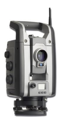
The Trimble® S8 Total Station serves both general surveying and specialized engineering applications. Ideal for one and perfect for the other, the flexible Trimble S8 Total Station with 1" angular accuracy and EDM precision of 1 mm + 1 ppm seamlessly switches between different project types. Always working, it secures your investment and ensures a fast return.
