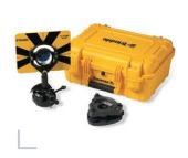
Contains case, traverse prism, prism base (with level and optical plummets) and tribrach (with no plummet). The prism base with level has a lever arm with bottom notch measurement that enables accurate height measurements and removes the need to remeasure when pairing with an S-series or SX instruments.
