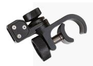
This part is compatible with both the TSC5 pole mount bracket and the TSC7 pole mount bracket. The attachable arm includes 3 options for attaching to the pole mount bracket. The pole clamp part (with the bracket/arm and TSC5 detached) remaining on the pole fits inside a 10 cm (4") tube.
