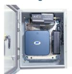
Monitoring cabinet to house the Settop M1 with UPS and charger. All accessories of the Settop M1 fit in this small waterproof box for quick access.
