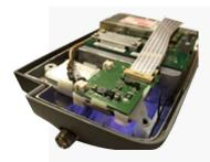
The Trimble Sentinel hardware module and application gives you real time tracking based on time or distance and allows you to easily locate lost, stolen or missing equipment. This is a service part upgrade for any \$5/\$7/\$9/\$9HP instrument and needs to be paired with the Trimble Sentinel subscription (103500-00).
