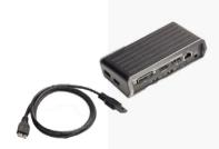
The desktop hub includes a USB cable and power supply. It connects to the TSC5 controller with the USB cable.
