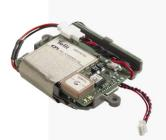
The Trimble Sentinel hardware module and application gives you real time tracking based on time or distance and allows you to easily locate lost, stolen or missing equipment. This is a service part upgrade for any Trimble C5 instrument and needs to be paired with the Trimble Sentinel subscription (103500-00).
